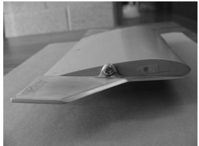
Fig. 5 View from starboard tip of MTS4A-2b set at ds = -5^\circ .
