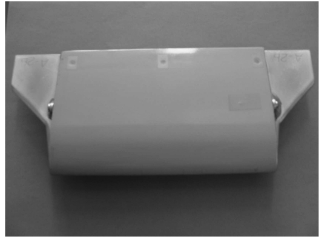
Fig. 3 Strakes MTS4A-2b attached to main wing.
